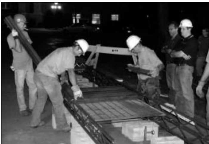
The LSU ASCE Student Chapter steel bridge team members participating in the proof loading of their competition bridge.
