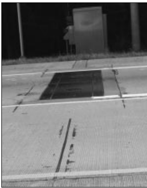
Figure 6. The WIM scale in the outside lane of the first gauntlet is shown with the cabinet that houses the computer on the gauntlet located on the shoulder. The piezoelectric axle sensor shown in the inside lane (foreground) is used to measure the axle spacing to determine the legal weights of vehicles that bypass the WIM scale.
