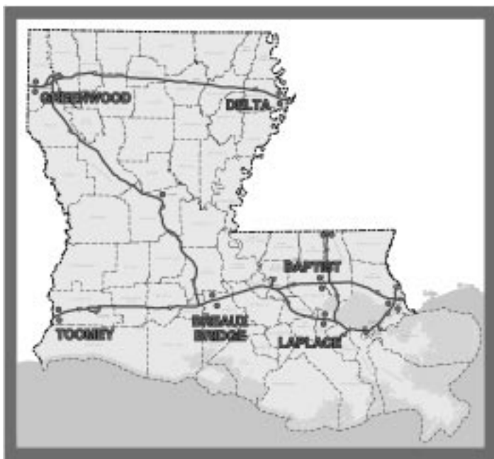
Figure 1 (left). Map of Louisiana showing the locations of the truck weight enforcement scales on the Interstate highway system that have AVI systems and existing or planned WIM systems. Figure 2 (above). A schematic diagram showing the location and the components of the three technology gauntlets for the WIM and AVI systems and a brief explanation of their functions.
