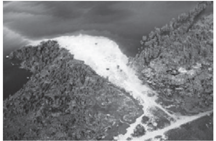
Figure 8. Sediment-laden channel water resulting in a sediment plume in the receiving lake water. (Courtesy of USDA Natural Resources Conservation Service.)
