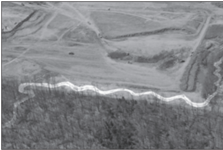
Figure 13. Example of a stable reference reach in equilibrium that could be used in the analog design approach.
