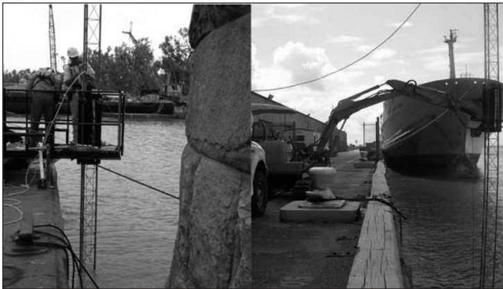
Figure 5 – Fenstermaker's self-contained LARS (Launch & Recovery Systems)
