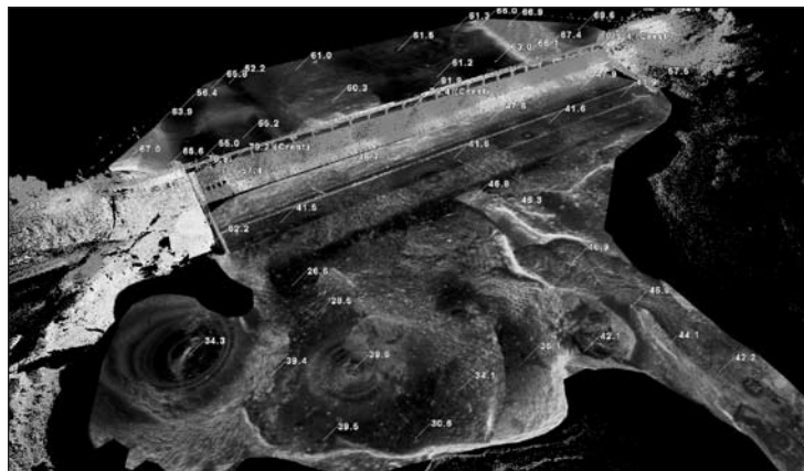
Figure 7 - Underwater Acoustic Imagery and spot profile elevations extracted from 3D model of integrated Underwater Acoustic Imaging and Profiling data and HDS Laser Scanning Data
