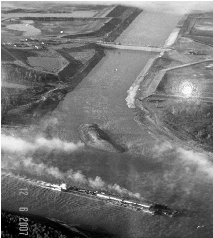
Figure 1- General view of the Sidney A. Murray Jr. Hydroelectric Station. The Island (ref: 1) at the entrance of the intake channel plays an important role by establishing uniform flow distribution downstream, which was essential for obtaining high plant efficiency. This channel compared to the Corps Low Sill or Auxiliary intake channel has no bank scour or sand deposition problems.
