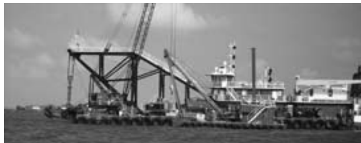
Figure 3. Cutter Head Dredge Alaska
