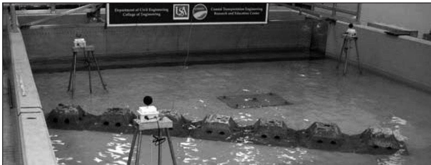
Figure 1. Laboratory testing of wave transmission through concrete wave attenuation devices in the USA CTEREC wave basin
