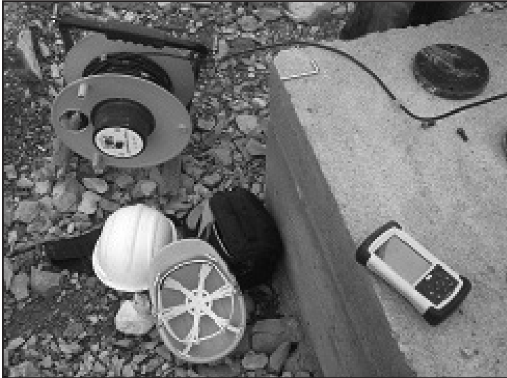
Manual measurement of inclinometer system (source: google images)
