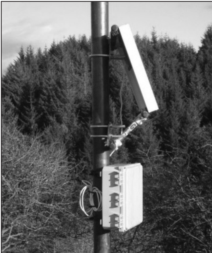
Wireless transmission of data from instruments (source: google images)
