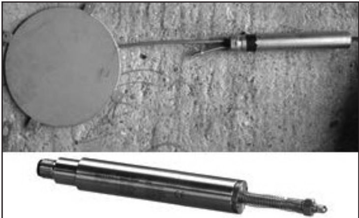
Earth Pressure Cell (top) and LVDT (bottom)
