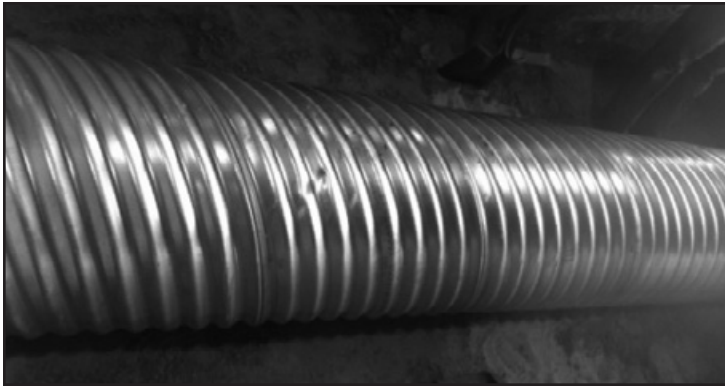
Culvert Positioned inside the Soil box
