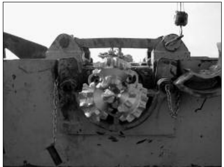
Figure 8. End view of the drill bit oriented with its 2 open mud jets located at the top and its plugged mud jet located at the bottom.
