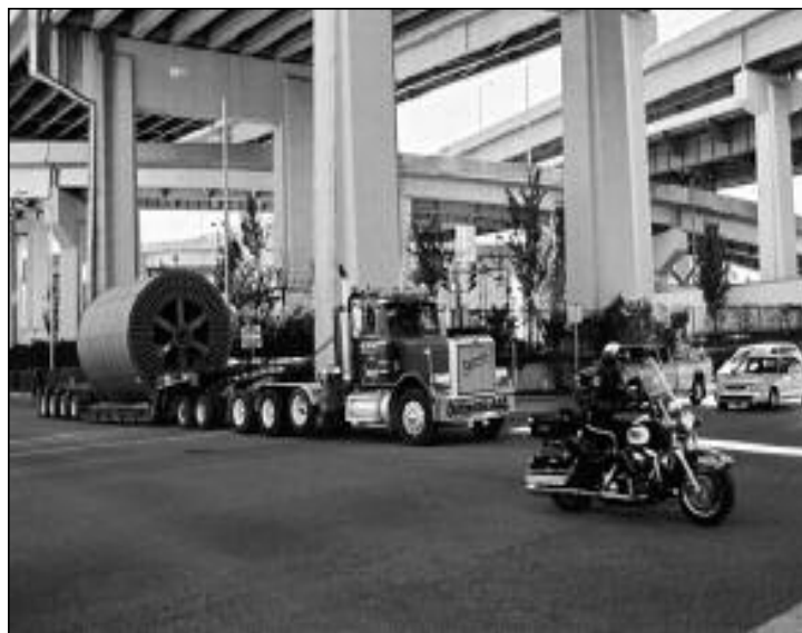
Figure 17. Truck transporting one of the 72-ton cable reels from the Port of New Orleans to the east bank site.
