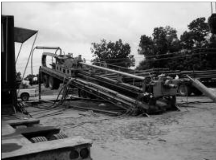
Figure 7. Trailer mounted HDD rig shown in position to begin drilling operations.
