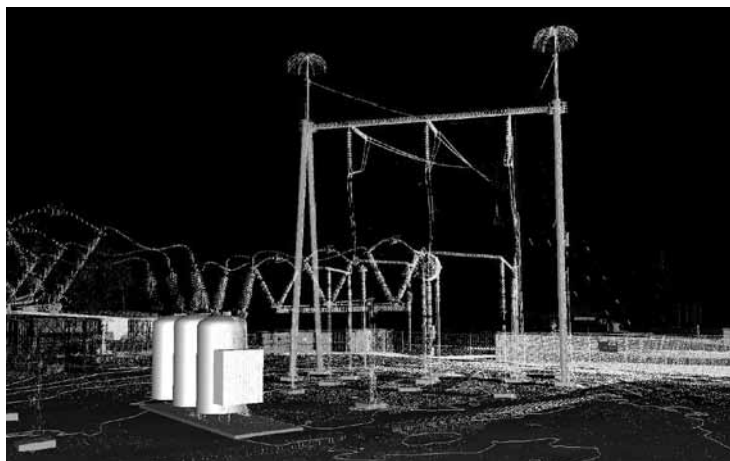
Figure 2: Point Cloud data of Electrical Substation
