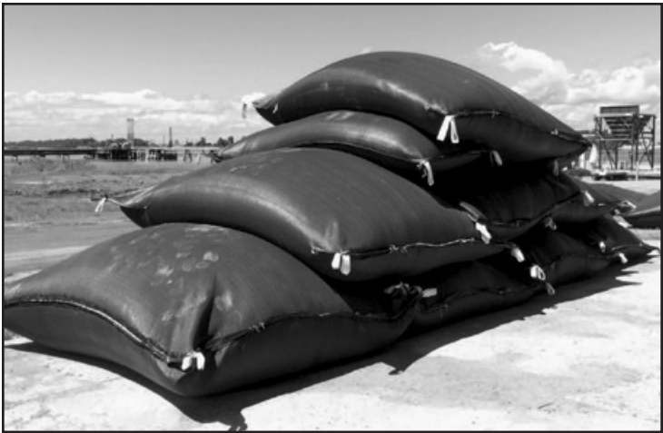
Figure 3: Filled lightweight aggregate bags ready for loading onto barge
